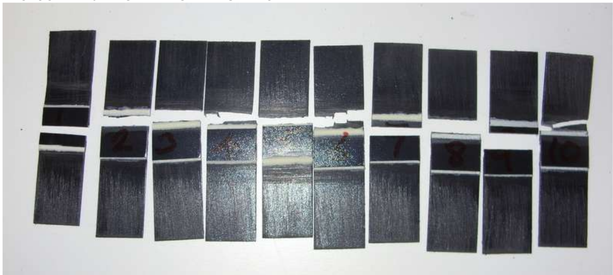
PHOTOGRAPH 3:- TEST PIECES – FAILURE MODE
